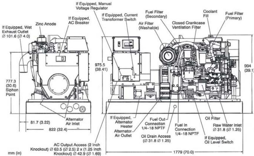
**Note:** This outline drawing is provided for general reference only and is not intended for design or installation. For more information see Operation and Installation manuals or obtain drawing 500-3799 and wiring diagram from your distributor/dealer.
