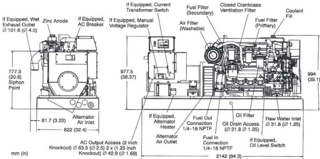
**Note:** This outline drawing is provided for general reference only and is not intended for design or installation. For more information see Operation and Installation manuals or obtain drawing 500-3800 and wiring diagram from your distributor/dealer.
